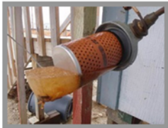
Free Water Ice Crystals Creates Abrasive Wear In Fuel System
